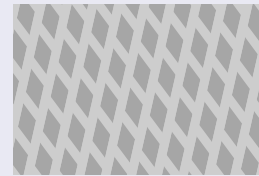
Diamond-shaped lubricant reservoirs
