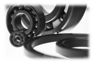
Silicon Nitride is the material of choice for vacuum and high speed rolling element applications. 58% lighter than traditional steel, Silicon Nitride provides a weight saving benefit. Due to reduction in weight, there is a reduction in centripetal force generated by the rolling elements. When used in similar applications and compared to bearing steel, Silicon Nitride offers a significantly increased fatigue life time.
