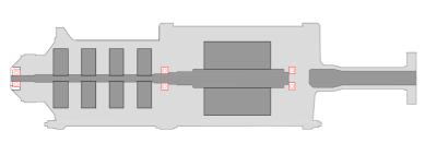
orientation immersed in a cryogenic liquid such as liquid Argon or Nitrogen at operating temperatures of between 155° to -196°C. An angular contact bearing pair was designed with Stainless Steel Races, Silicon Nitride Ceramic Balls and a custom PEEK Cage. The UNASIS XTRTD dry film lubrication was also applied to meet with the demand of extreme low temperature, extremely high loading and speed conditions.
