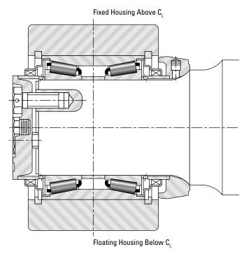
Fig. 13 Cross section of AP bearing in housing
