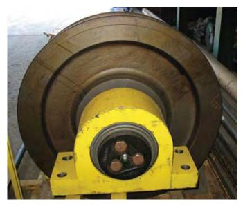
Fig. 12 AP bearings used in pillow block application
