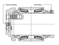
Fig. 41 Mounting Arrangment 3-B
