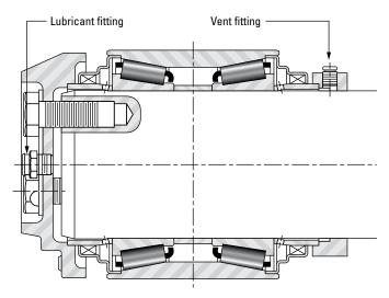
Fig. 32 Cross section view of AP bearing
