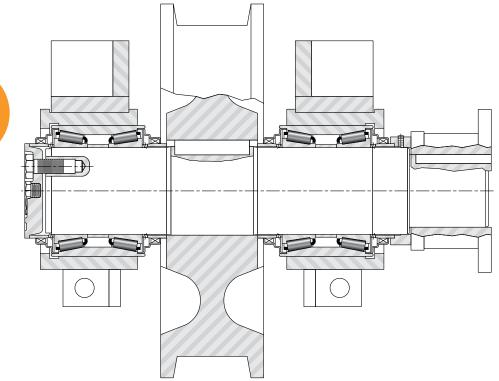
Fig. 3 Cross section of AP bearing on a drive axle
