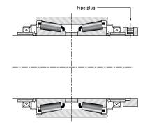
Fig. 45 Mounting Arrangment 5-A
