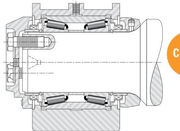
Fig. 22b Cross section of wood pulp beater spindle
