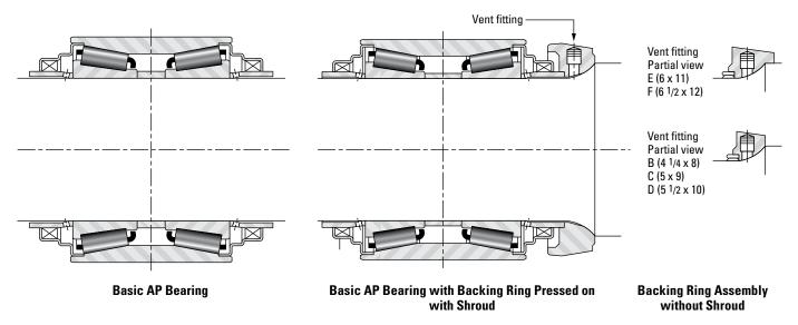
NOTE: Specify backing ring with or without shroud. Backing rings without shroud have reduced 0.D. to facilitate assembly in some housing designs. Backing rings with shroud provide added seal protection where required.
