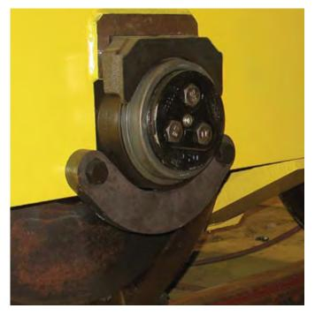
Fig. 8 Narrow adapter mounting on trolley safety bar
