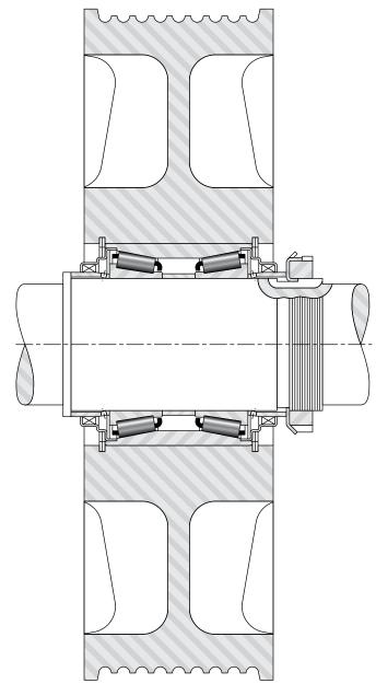
Fig. 14 Section view of elevator sheave
