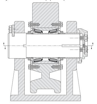
Fig. 23 Furnace wheel
