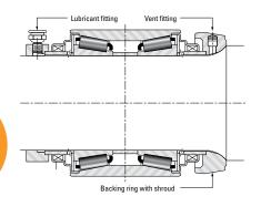
Fig. 37 Mounting Arrangment 2-A
