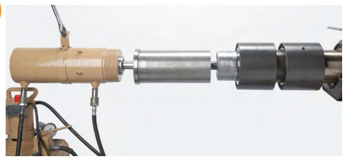
Fig. 28 Tooling used to push bearing onto shaft
