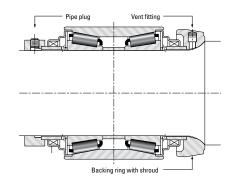
Fig. 38 Mounting Arrangment 2-B
