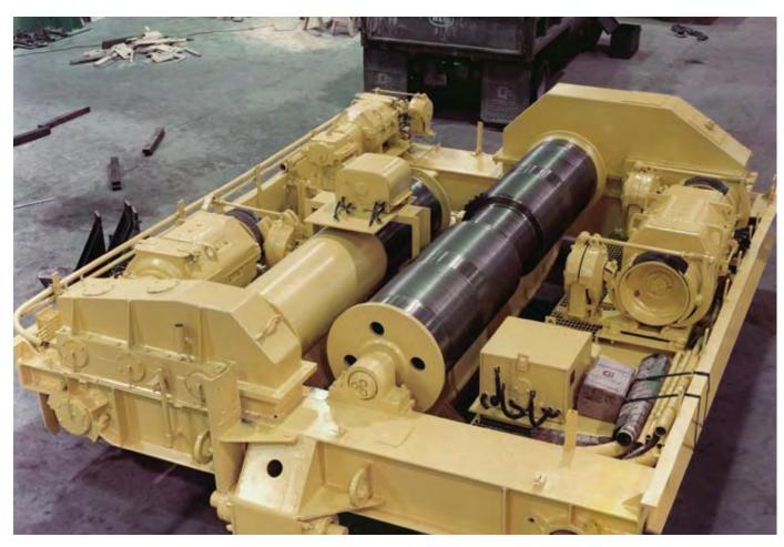
Fig. 6 Trolley utilizing AP bearings with recessed end cap for wheel and drum drive
