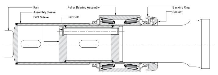
Fig. 26 Separate sleeve method of applying roller bearings to a shaft
