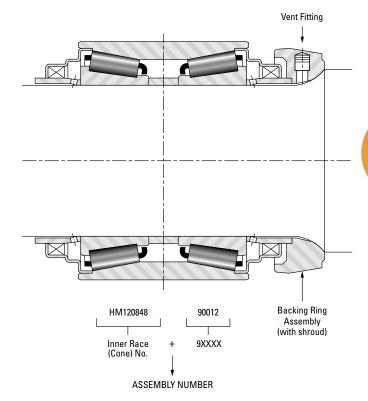
Fig. 2 Typical AP bearing assembly
