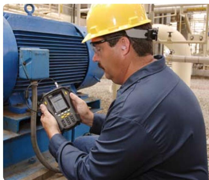
*SKF Microlog series data collectors/analysers*
