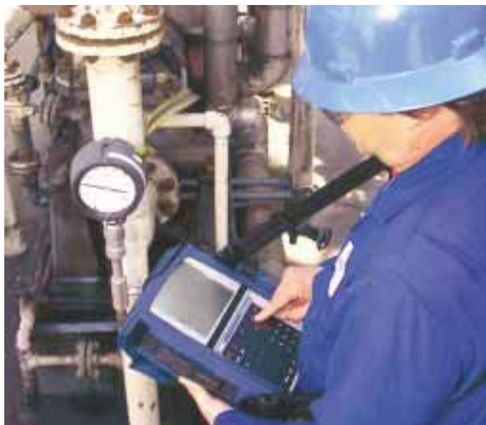
Microlog – portable data collector and analyser
