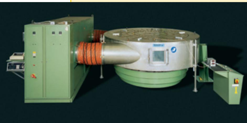
Frictional torque measurement at sub-zero temperature in the climatic test chamber
