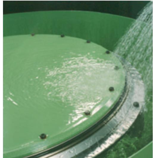
Tightness test ("splash water test") of a wire-race bearing with integrated slip rings for electric current transmission (see page 8, fig. 14)
