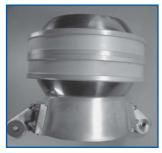
**5.** Main Rotor Swashplate Slider Bearings
