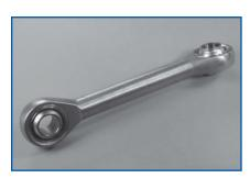
2. Tail Rotor Pitch Link Bearings
