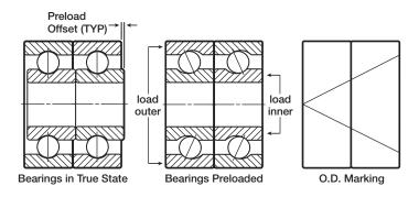
With tandem (DT) pairs, both inner and outer rings abut and are capable of sharing a thrust load, providing increased thrust capacity.
