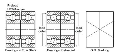
When face-to-face (DF) duplex pairs are mounted, the inner rings abut and the outer rings are drawn together, providing a higher radial and axial stiffness and accommodation of misalignment.
