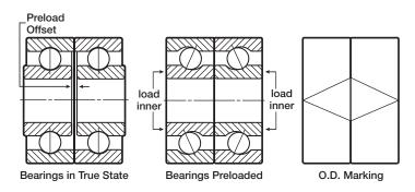
When a back-to-back (DB) duplex pair is mounted, the outer rings abut and the inner rings are drawn together, providing maximum stiffness.
