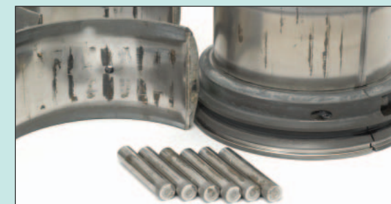
Fig. 16 Rust on Bearing Supporting Roll at Middle Position
