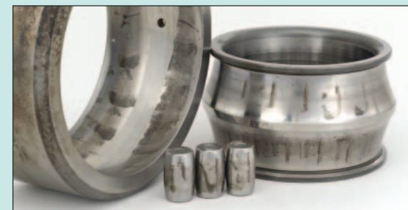
Fig. 15 Rust on Spherical Roller Bearing Caused by Water Ingress
