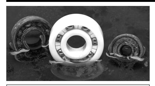
STEEL BEARINGS CORRODE IN LIQUIDS
