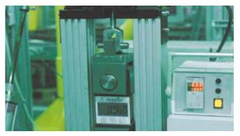
Test bench for loads up to 150 MPa and temperatures up to +250 °C
