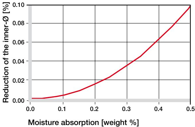
**Diagram 11: Effect of moisture absorption plain bearings****Installation Tolerances**
