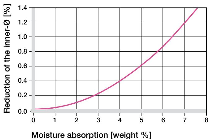
Diagram 10: Effect of moisture absorption on plain bearings
