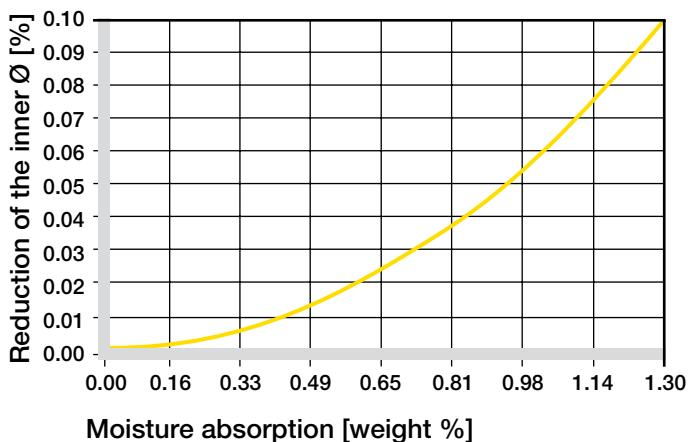
**Diagram 10: Effect of moisture absorption on plain bearings**
