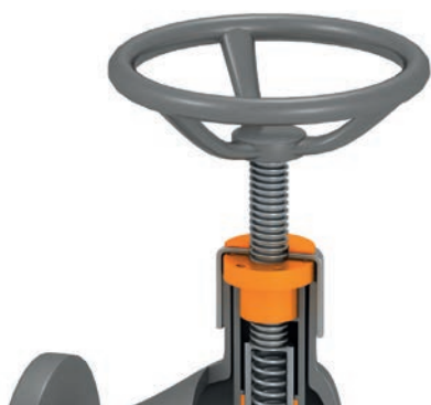
Lead screw nut in block valve
