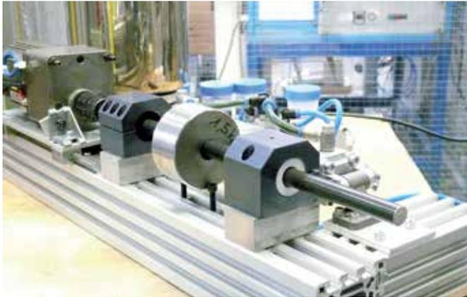
Test bench for xiros® polymer ball bearings at igus® laboratory
