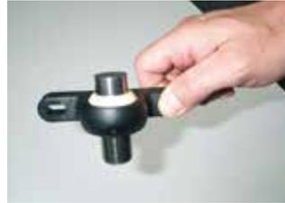
**Tolerance test with gauge**
