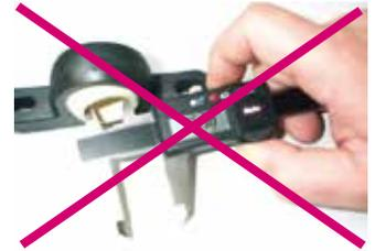
**Wrong test equipment; caliper**
