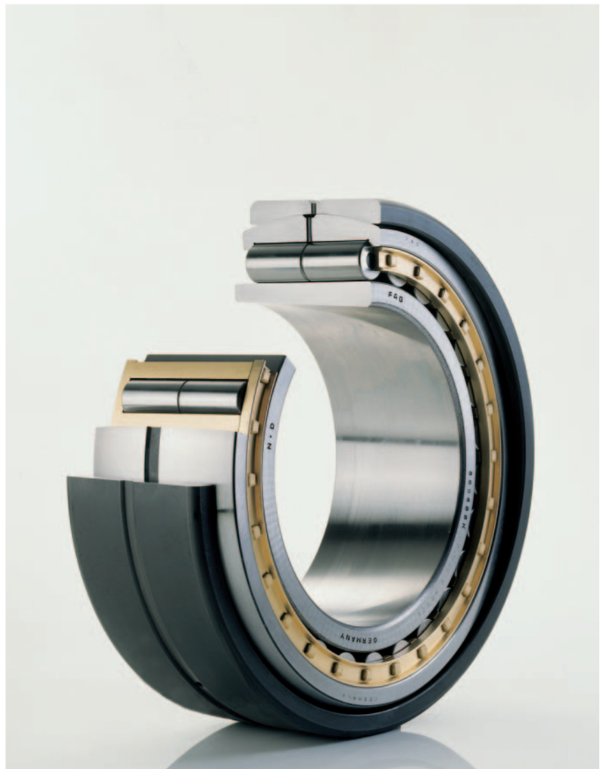
3: Self-aligning cylindrical roller bearings are ideal non-locating bearings for dryer rolls, M.G. cylinders and guide rolls. Lubrication grooves and lubrication holes in the outer ring and plain bearing pivot ring allow lubricant feed directly to the rolling contacts.
