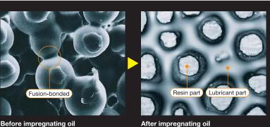
After impregnating oil (Capillary lubrication structure)
