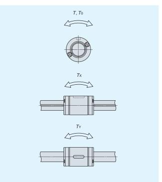
Fig.2 Direction of dynamic rated torque, static rated torque and static rated moment
