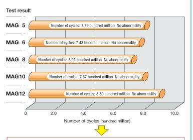
At vertical shaft and super high tact operation, the product can endure at the total number of reciprocating motions of 2 hundred million without any trouble only with the oil prepacked in the C-Lube.
