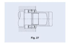
When press fitting, the friction of the fitting surfaces can be reduced by applying high viscosity oil over the fitting surfaces.
