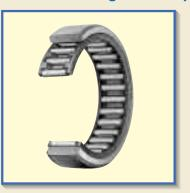
In Needle Roller Bearings with Separable Cage, the inner ring, outer ring and Needle Roller Cage are combined, and they can be separated easily. This type has a simple structure with high accuracy. In addition, the radial clearance can be freely selected by choosing an assembly combination.
