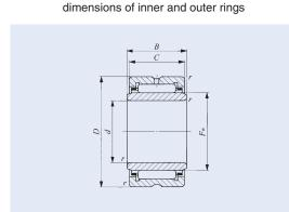
Fig. 7 Machined Type Needle Roller Bearing
