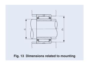
unit: mm  $r_{\rm s \, min}$  $r_{\rm as\ max}$ Largest permissible single Smallest permissible single chamfer orner radius of shafts and dimension housings 0.1 0.1 Housing 0.15 0.15 0.2 0.2 0.3 0.3 0.4 0.4 0.6 0.6 1 1.1 1 1.5 1.5 2 2 Shaft 2.1 2 2.5 2 3 2.5 4 3 5
