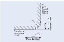
Fig. 12 Permissible values for chamfer dimensions
