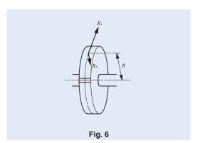
In this case, the resultant normal force on the tooth surface acts as the radial force to the shaft and the magnitude of vibration or shocks varies depending on the accuracy and surface finish of the gear. Therefore, the radial load  $K_{\rm r}$  applied to the shaft is obtained from the following equation, multiplying the resultant normal force  $K_{\rm c}$  on gear tooth surface by the gear factor  $f_{\rm z}$  shown in Table 8.
