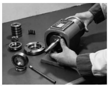
FIGURE 5 - MOUNTING DRIVE-END BEARINGS
