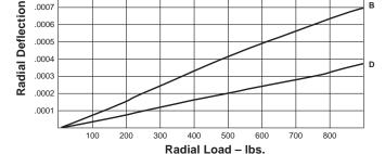
B Preloaded DBD Preloaded Tandem
