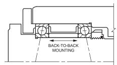
Figure 6 - DB Mounting, Fixed
