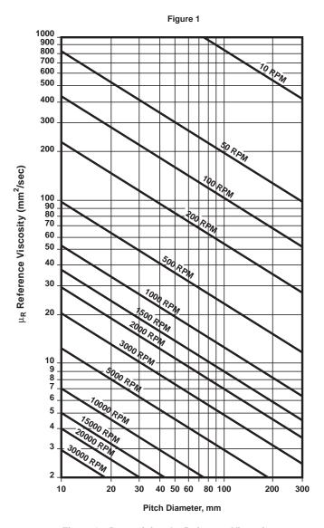
Figure 1 – Determining the Reference Viscosity
