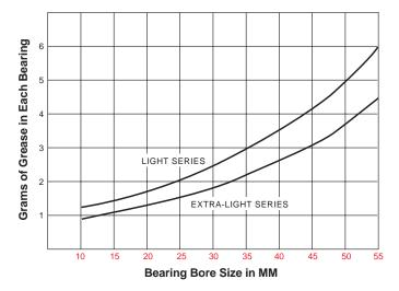
Figure 17 - Grease Quantity Chart
