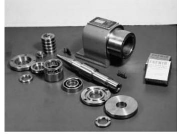
Figure 3 - Wheelhead Parts
