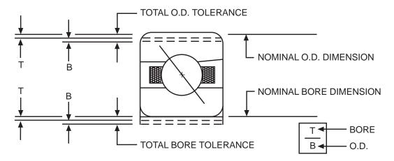
Offering bore and O.D. coding makes it easier to obtain the optimum recommended fits for spindles. Each bearing in a set is matched to within half the bore and O.D. tolerance to insure equal load sharing. It also enables our customers to use pairs of bearings with same bore and O.D. codes to make triplex and quadruplex sets.
