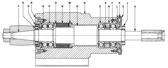
Figure 1 - Internal Grinding Wheelhead
