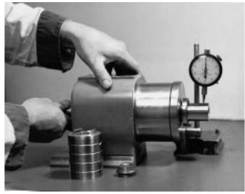
Figure 6 - Checking Nose-End Runout
