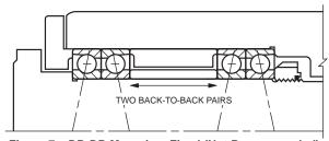
Figure 7 – DB-DB Mounting, Fixed (Not Recommended)
