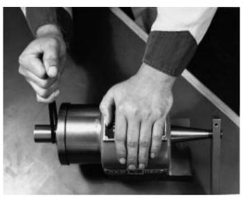
Figure 7 - Tightening with Spanner Wrench
