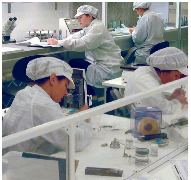
All Barden precision bearings are assembled under stringent clean room conditions.
